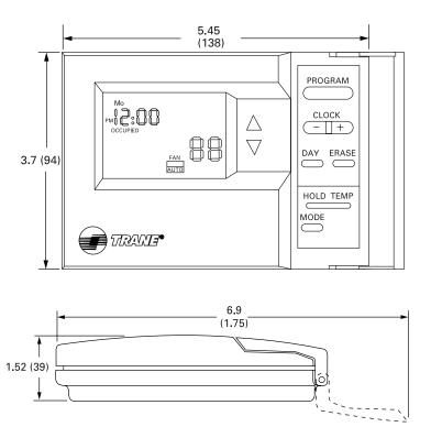
Field Installed Sensors Constant and Variable Air Volume
